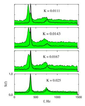
**Fig. 9.18.** (Color online) Evolution of the power spectrum obtained from electronic experiment. This figure illustrates a transition via the suppression of the noise-induced frequency in the driven system
