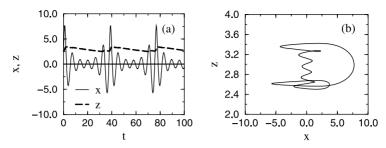
**Fig. 12.15.** Self-modulated regime 1:6 in a single Anishchenko–Astakhov oscillator (12.17): a realization and **b** phase portrait at m = 2.90328, g = 0.012505, and  $b = 5 \times 10^{-5}$
