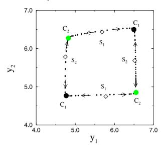
**Fig. 12.13.** (Color online) Poincaré section of the resonant torus for two coupled Rössler models (12.1). The secant was chosen as  $x_1=0$ . Control parameters are  $\alpha=0.15$ ,  $\beta=0.2$ ,  $\mu=5.0$ , and  $\gamma=0.0273$ . Points  $C_{1,2}$  denote the stable limit cycles while  $S_{1,2}$  are the saddle cycles. *Arrows* indicate the stable directions along the resonant torus surface
