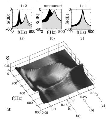
**Fig. 13.9.** Two-mode collective response in the system of two monovibrators mutually coupled as shown in Fig. 13.7(b), at  $D=0.475~\rm V^2$  and different g. The evolution of the power spectrum S(f) clearly shows the transitions from a 1:2 frequency-locking (g=0.18) to **b** non-resonant two-mode behavior (g=0.25), and finally to **c** 1:1 mode locking (g=0.325); **d** three-dimensional plot illustrating frequency entrainment with varying coupling strength
