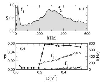
Fig. 13.14. Two-mode dynamics in the excitable system presented in Fig. 13.13(a). a Power spectrum of the sum of the outputs of two units; note well-pronounced peaks ( $D = 0.34 \text{ V}^2$ ). b Peak frequencies (*empty circles*) and regularity  $\beta$  (*filled circles*) vs noise intensity D
