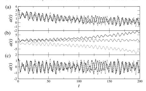
**Fig. 7.2.** Illustrations of various random processes. In each panel a, b or c three realizations of the same random processes are shown, launched from the same initial conditions. a Random process whose average value changes in time. b Random process whose variance changes in time. c Stationary random process
