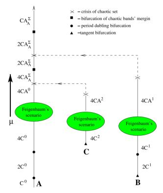
Fig. 12.6. (Color online) Evolution of oscillatory regimes in coupled Rössler systems (12.1) at frequency mismatch  $\Delta=0.0093$
