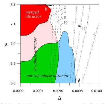
**Fig. 12.8.** (Color online) Bifurcation diagram near the boundary of synchronization region of coupled Rössler systems (12.1). *Dashed* and *dotted curves* denote bifurcations of periodic orbits on branches **A** and **B**. Numbers 2, 4, and 8 denote the periods of saddle cycles
