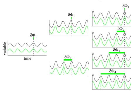
**Fig. 12.1.** (Color online) Schematic representation of different phase relations between oscillations corresponding to period-one (**left panel**), period-two (**middle panel**) and period-four limit cycles (**right panel**). The oscillations in the first and the second systems are denoted by *black* and *grey solid curves*, respectively. The *dashed lines* of the corresponding colors indicate the positions of the largest maxima of oscillations
