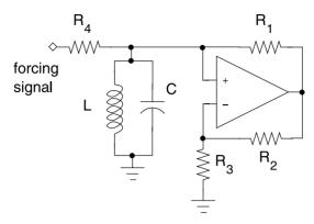
**Fig. 3.13.** Scheme of an experimental setup used to illustrate the phenomena of forced synchronization. The LC-oscillator is used with the following circuit parameters:  $R_1 = R_2 = 1.5 \,\mathrm{kOhm}$ ,  $R_3 = 40 \,\mathrm{Ohm}$ ,  $R_4 = 50 \,\mathrm{kOhm}$ ,  $L = 18 \,\mathrm{mH}$ ,  $C = 33 \,\mathrm{nF}$ . The frequency  $f_0$  of self-sustained oscillations in this circuit was measured to be equal to  $6.62 \,\mathrm{kHz}$
