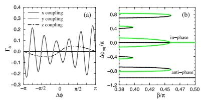
**Fig. 12.16.** (Color online) Phase analysis of the self-modulated regime of coupled Anishchenko–Astakhov oscillators (12.18). **a** Antisymmetric part  $\Gamma_a$  of effective coupling function; **b** Evolution of location and stability of coexisting regimes when the coupling vector is gradually changed from  $K_x$  to  $K_z$ . *Black circles* denote stable solutions
