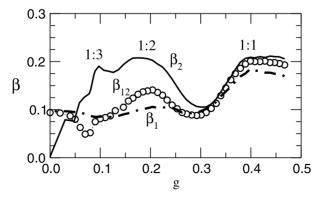
**Fig. 13.11.** Measures of regularity as a function of coupling strength ( $D = 0.475 \text{ V}^2$ ) for the first ( $\beta_1$ ) and second ( $\beta_2$ ) units, and for their collective response ( $\beta_{12}$ )
