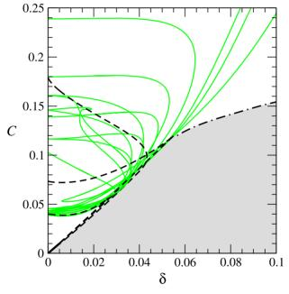
**Fig. 8.31.** (Color online) The vicinity of synchronization region for two coupled Rössler oscillators (8.15). *White area* outlines synchronization region. Bifurcations of unstable limit cycles are indicated by lines: *black dashed lines*—saddle-node bifurcations; *black dot-dashed line*—Neimark—Sacker bifurcation; *grey solid lines*—period-doubling bifurcations
