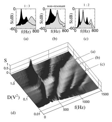
**Fig. 13.10.** Two-mode collective response in the system of two monovibrators mutually coupled as shown in Fig. 13.7(b), at g=0.1. Spectrum is shown at different D: **a** 1:3 frequency-locking ( $D=0.77~\rm V^2$ ); **b** non-resonant two-mode behavior ( $D=0.42~\rm V^2$ ); **c** 1:2 mode locking ( $D=0.15~\rm V^2$ ); and **d** three-dimensional plot illustrating frequency entrainment with varying coupling strength
