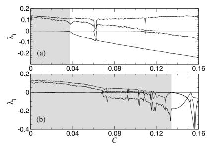
**Fig. 8.32.** Synchronization transitions in terms of Lyapunov exponents in (8.15). Four largest Lyapunov exponents are given as functions of C at **a**  $\delta = 0.02$  (locking), **b**  $\delta = 0.07$  (suppression). White areas correspond to synchronization regions
