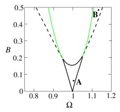
**Fig. 7.7.** (Color online) The vicinity of 1:1 synchronization region of a forced van der Pol system as described by (7.116) with  $\lambda = 0.2$ . *Solid lines*: saddle-node bifurcations; *dashed*: torus birth
