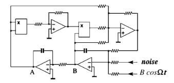
Fig. 7.15. Scheme of electronic circuit modelled by (7.116)
