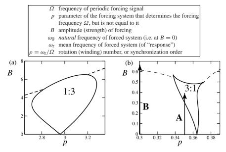
**Fig. 6.5.** Bifurcation diagrams in the vicinities of **a** 1:3 and **b** 3:1 synchronization regions in a van der Pol oscillator forced by another van der Pol oscillator (6.2)–(6.3) at  $\lambda = 0.5$ . *Solid black lines*: saddle-node bifurcations; *dashed lines*: torus birth bifurcations
