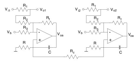
Fig. 9.2. The electrical scheme for the coupled monovibrator circuit. Both units are identical but the noise sources  $(V_{i1} \text{ and } V_{i2})$  are independent
