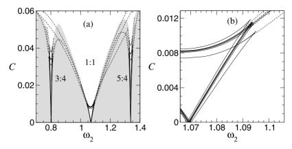
**Fig. 8.22.** a Region of synchronization of periodic oscillations by chaotic forcing (*white area*) in (8.13)–(8.14), which is defined from (8.9). **b** Zoomed part of **a**. Lines are bifurcations of unstable limit cycles embedded in the chaotic attractor: *solid lines*—saddle-node bifurcations, *dashed*—Neimark–Sacker (torus birth/death) bifurcations
