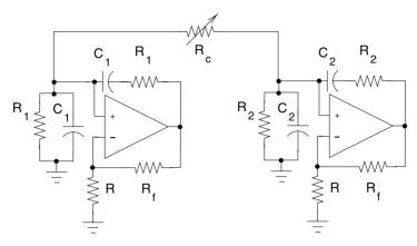
**Fig. 4.11.** Scheme of an experimental setup used to illustrate the phenomena of mutual synchronization. The Wien bridge oscillators are used with the circuit parameters as follows: **Locking**:  $R_1 = R_2 = 1.5 \text{ kOhm}$ ,  $R_f = 20 \text{ kOhm}$ , R = 9 kOhm.  $C_1 = 33 \text{ nF}$ ,  $C_2 = 35 \text{ nF}$ , **Suppression**:  $R_1 = 1.5 \text{ kOhm}$ ,  $R_2 = 1.65 \text{ kOhm}$ ,  $R_f = 20 \text{ kOhm}$ ,  $R_f = 9 \text{ kOhm}$ ,  $R_f = 20 \text{ kOhm}$ ,  $R_f = 2$
