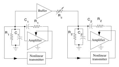
**Fig. 8.8.** Scheme of an experimental setup used to illustrate the phenomena of chaos synchronization. Two Anishchenko–Astakhov oscillators are coupled unidirectionally via a buffer
