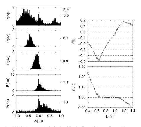
**Fig. 9.13.** Stochastic synchronization in unidirectionally coupled monovibrators (electronic experiment). **Left panels**: The phase difference distribution with increasing of  $D = D_1$ . **Right top panel**: Mean phase difference. **Right bottom panel**: The evolution of frequency ratio
