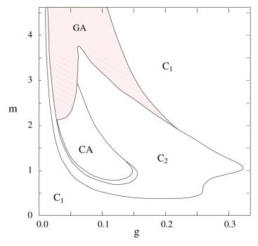
**Fig. 13.16.** (Color online) Map of regimes for the system (13.17) on the parameter plane (g, m).  $C_1$  is an area of existence of a period-one limit cycle;  $C_2$  is a domain of period-two limit cycle; CA is a region of chaotic attractor resulting from a cascade of period-doubling bifurcation; GA is an area where the system demonstrates complex oscillations accompanied by a drift in y-direction
