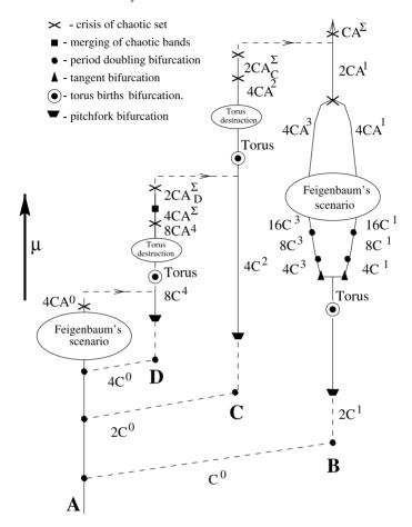
**Fig. 12.2.** Evolution of oscillatory regimes for the identical coupled Rössler systems. The *solid* and *dashed lines* correspond to bifurcational transitions of attractive and saddle solutions, respectively
