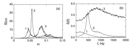
**Fig. 9.4.** The evolution of power spectra **a** for the noise-driven Morris–Lecar model (curves I, 2, and 3 in **a** correspond to D = 0.0001, 0.001, and 0.01  $V^2$ , respectively) and **b** for the noise-driven monovibrator circuit (curves I, 2, and 3 in **b** correspond to D = 0.015, 0.1, and 0.6  $V^2$ , respectively)
