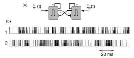
**Fig. 13.13. a** Two monovibrators with delayed inhibitory couplings imitate a simple neural circuit. **b** Stochastic spike trains generated by the first and the second excitable units. Antiphase behavior is registered in average
