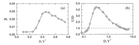
Fig. 9.6. Electronic experiment on monovibrator circuit. a Regularity  $\beta$  of noise-induced oscillations and b output power vs noise intensity D
