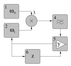
**Fig. 13.15.** Block diagram of a phase-locked loop: I—generator of a reference signal with frequency  $\omega_0$ ; 2—generator with controlled frequency  $\omega_1$ ; 3—phase detector; 4—low-pass filter; 5—amplifier; 6—non-linear feedback loop of the amplifier
