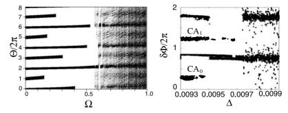
**Fig. 12.14. Left panel**: One parameter bifurcation diagram for the model map (12.9), (12.10) with K=0.5,  $\delta_i=0.45$ , B=1.2, and N=3. The figure shows how the coexisting noise inflicted periodic orbits one by one lose their synchronization. **Right panel**: One-parameter bifurcation diagram for two coupled Rössler systems (12.1) shows similar behavior for  $\alpha=0.15$ ,  $\beta=0.2$ ,  $\gamma=0.02$ , and  $\mu=6.7$
