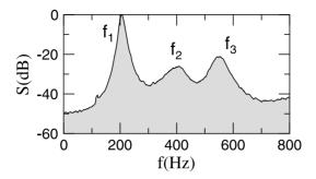
**Fig. 13.12.** Power spectrum illustrating three-mode collective behavior in a system of three interacting excitable units sketched in Fig. 13.7(c) at  $D=0.35~\rm V^2$  and g=0.03. Peak frequencies are estimated as  $f_1=205.3~\rm Hz$ ,  $f_2=403.5~\rm Hz$ , and  $f_3=549.1~\rm Hz$
