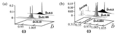
**Fig. 7.16.** Spectra measured in a full-scale experiment with van der Pol circuit (Fig. 7.15). **a** 1:1 phase locking; **b** 1:3 phase locking
