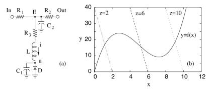
**Fig. 14.7.** a Circuit diagram and **b** the nullclines for the 2D limit case  $R_{1,2} = 0$ . In the dimensionless model equations (14.11), x represents the voltage u across the tunnel diode D, y is the current i in the inductor L, and z is the voltage E across the capacitor  $C_2$
