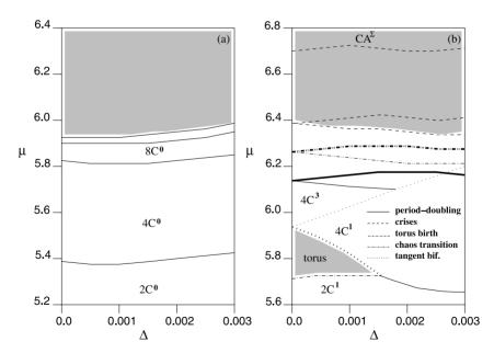
**Fig. 12.5.** Bifurcation diagram on  $(\Delta - \mu)$  parameter plane of the system (12.1) for the attractors of branches **A** (a) and **B** (b). Curves of different width correspond to different families of attractors
